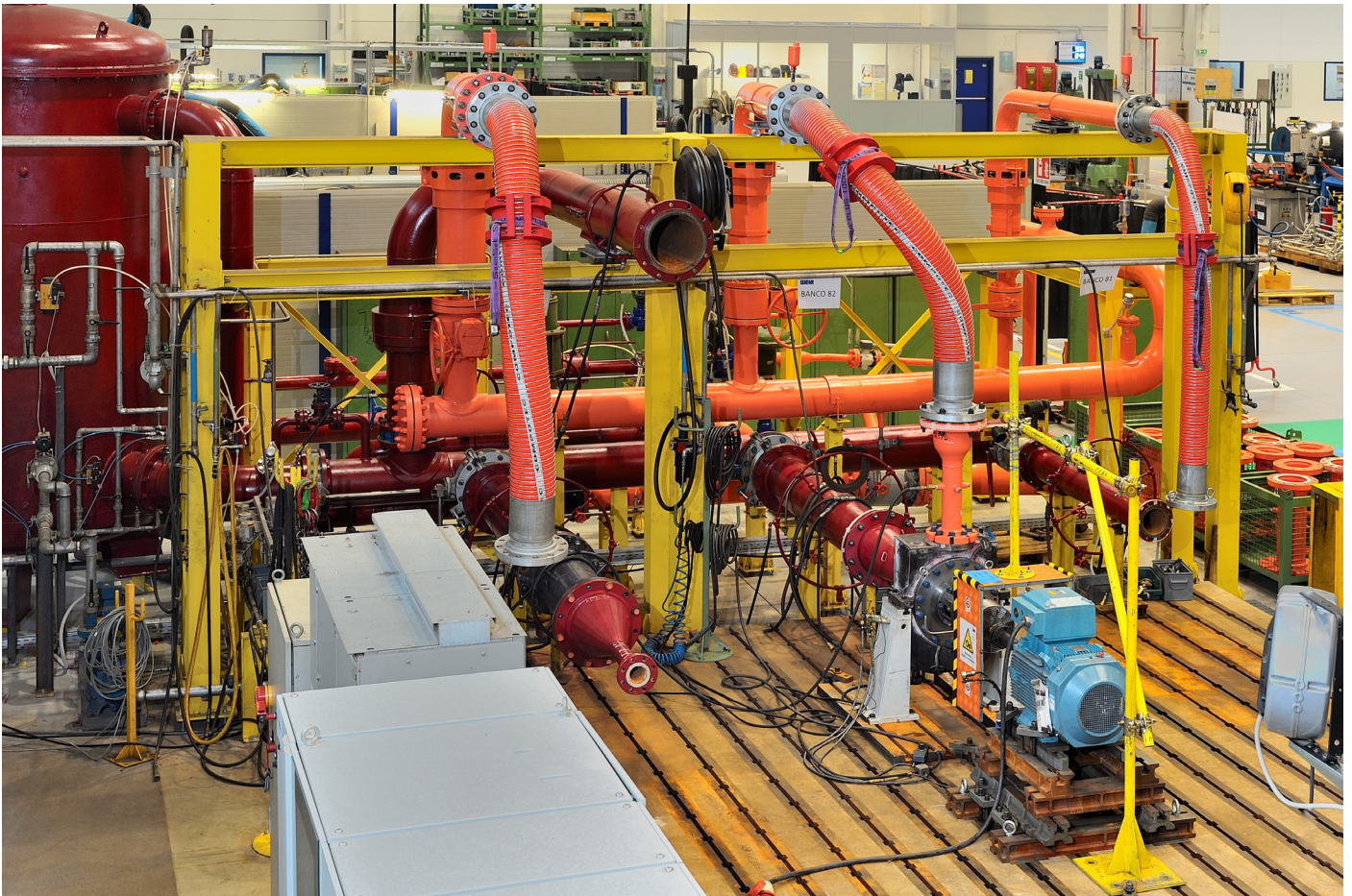
Gabbioneta Test Room – R pumps benches
