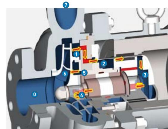
Fig.2. Pressure / temperature profile / isolation shell flush flow
