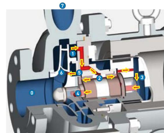
Fig.1. Pressure / temperature profile / journal bearing flush flow
