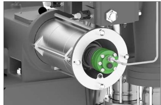
Fig. 9: The extended piston rod can serve as piston compressor to ensure continuous filling of the air vessel.
