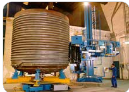
Automatized welding tool
