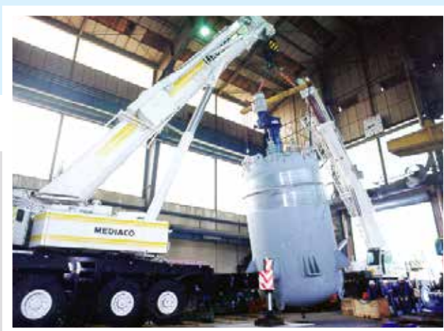
King size glass-lined reactor Handling 75 tonnes
