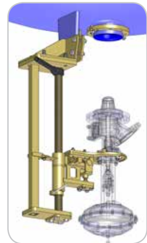
Alternative tool: fixed on the lifting lug
