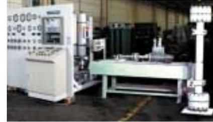
Valve test station for leak and functional tests at up to 5,000 bar
