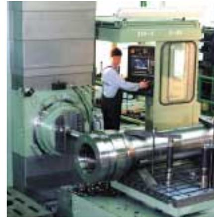
Machining of high pressure components on a boring mill with CNC in six axes
