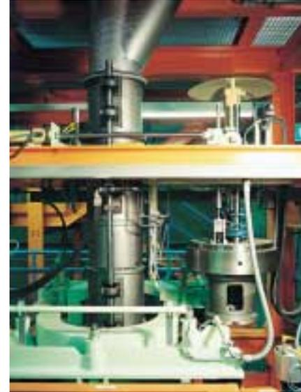
Autoclave with an automatic quick-acting clamp closure
