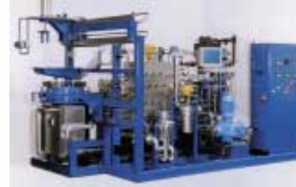
Pilot plant for dyeing synthetic fibres
