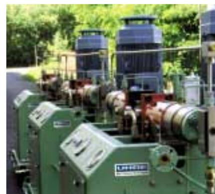
Catalyst injection pumps, 80 l/h, 3,000 bar
