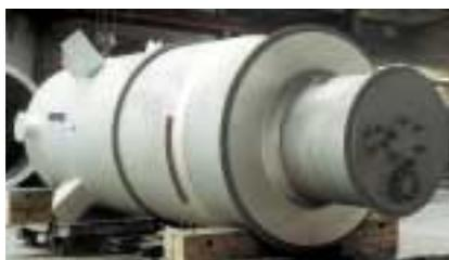
Separator, 18 m<sup>3</sup>, 440 bar, 350°C
