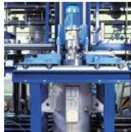
Stirrer-type reactor with a permanent-magnetic stirred drive (100 l, 300 bar)
