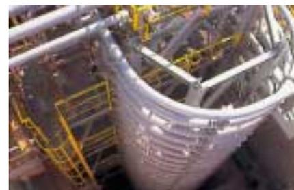
LDPE tubular reactor, DN 62 mm, 3,500 bar
